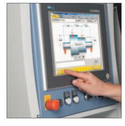
CAB 920, the 5<sup>th</sup> generation of digital balancing technology, provides you with perfectly balanced rotors and simple operation.
