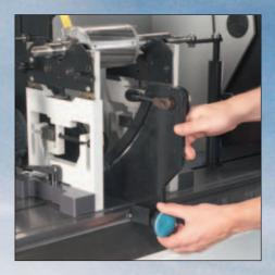
The belt drive can be adjusted to the correct rotor diameter in no time.
